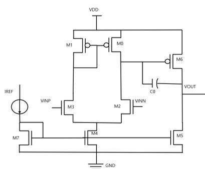
Fig. 1. Schematic Design of Two-stage Regulated Cascode Amplifier .
