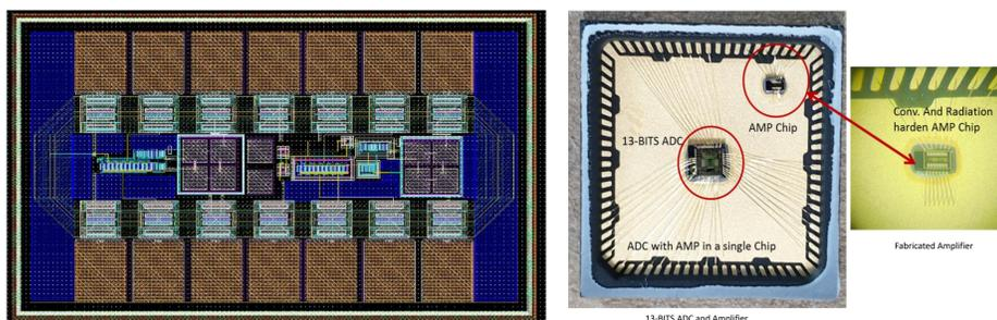
Fig. 2. . Layout Design of Two-stage Regulated Cascode Amplifier (Left) and Internal view of fabricated customized amplifier with analog to digital converter (ADC) on a same chip.
