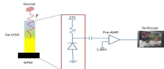
Fig. 3. Schematic illustration of Experimental Setup.
