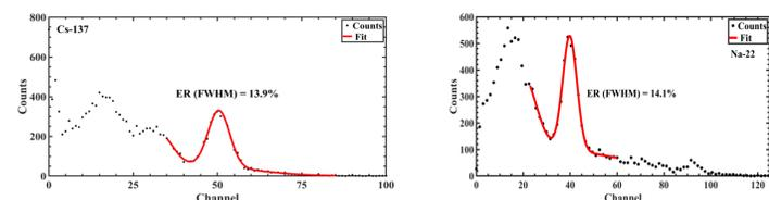
Fig. 3. Energy Resolution Spectrum for Cs-137 (Left) and Energy Resolution Spectrum for Na-22 (Right)
